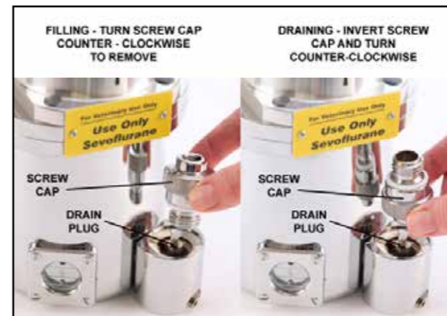
Fig 3. Filling and Draining – Screw Cap Filler
