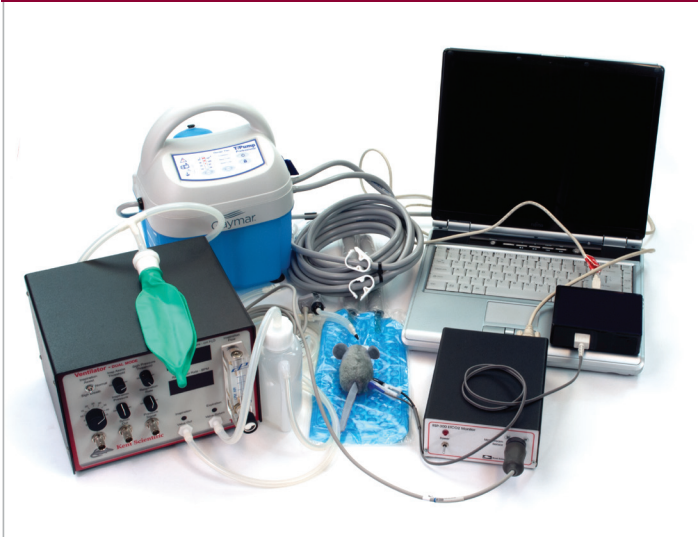
Image 1: Traditional monitoring devices for pulse oximetry, heart rate monitoring, artificial ventilation, ETCO 2 , and temperature monitoring and warming occupy significant bench space.
