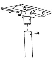
3) Use the included Hex Head Cap Screws to attach the mounting plate to the swivel/tilt head. Adjust the socket head screw to adjust the tilt tension.
